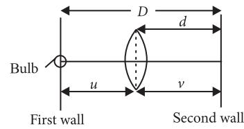
Now, we know that to form a real image of an object on a screen by a convex lens, the distance between the source and the screen ( $D$ ) should be equal to  $4f$ , where  $f$  is the focal length of the lens.In that case,  $u = v = D/2 = d$ .
